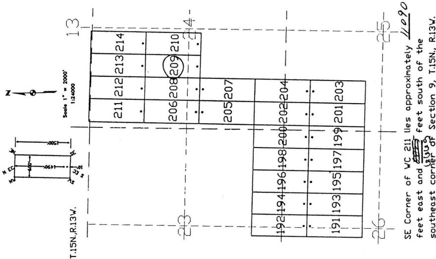
The above map depicts the WC 209 lode mining claim, which is located in Section (s) 24, Township 15 North, Range 13 West, Gila and Salt River Base Meridian, Mohave County, Arizona. The claim corners, end centers, and location monument are marked by 2 inch by 2 inch by 5 foot wooden posts with aluminum tags. The bearings and distances between claim corners are as depicted on the map.
