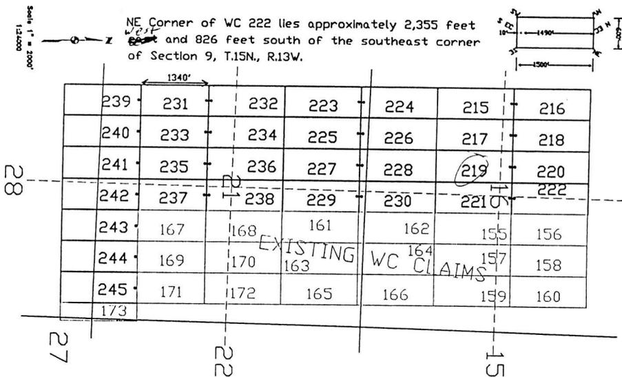
The above map depicts the WC 219 lode mining claim, which is located in Section (s) 16, Township 15 North, Range 13 West, Gila and Salt River Base Meridian, Mohave County, Arizona. The claim corners, end centers, and location monument are marked by 2 inch by 2 inch by 5 foot wooden posts with aluminum tags. The bearings and distances between claim corners are as depicted on the map.
