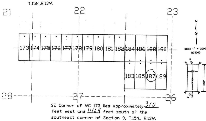
The above map depicts the WC 187 lode mining claim, which is located in Section (s) 20, Township 15 North, Range 13 West, Gila and Salt River Base Meridian, Mohave County, Arizona. The claim corners, end centers, and location monument are marked by 2 inch by 2 inch by 5 foot wooden posts with aluminum tags. The bearings and distances between claim corners are as depicted on the map.
