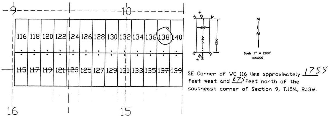
The above map depicts the WC 130 lode mining claim, which is located in Section (s) 10, Township 15 North, Range 13 West, Gila and Salt River Base Meridian, Mohave County, Arizona. The claim corners, end centers, and location monument are marked by 2 inch by 2 inch by 5 foot wooden posts with aluminum tags. The bearings and distances between claim corners are as depicted on the map.
