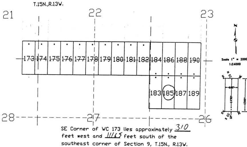
The above map depicts the WC 185 lode mining claim, which is located in Section (s) 26, Township 15 North, Range 13 West, Gila and Salt River Base Meridian, Mohave County, Arizona. The claim corners, end centers, and location monument are marked by 2 inch by 2 inch by 5 foot wooden posts with aluminum tags. The bearings and distances between claim corners are as depicted on the map.
