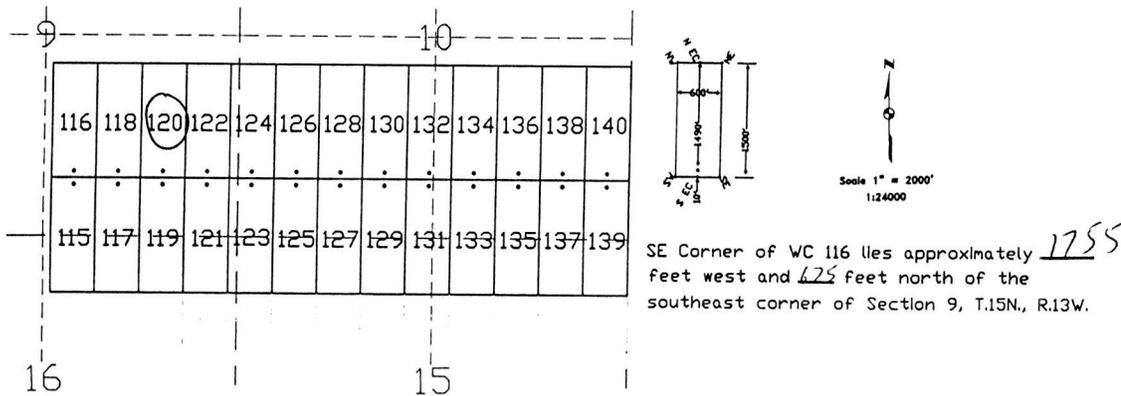
The above map depicts the WC 120 lode mining claim, which is located in Section (s) 9, Township 15 North, Range 13 West, Gila and Salt River Base Meridian, Mohave County, Arizona. The claim corners, end centers, and location monument are marked by 2 inch by 2 inch by 5 foot wooden posts with aluminum tags. The bearings and distances between claim corners are as depicted on the map.
