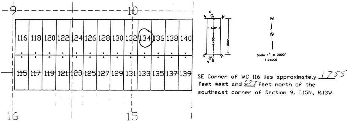
The above map depicts the WC 134 lode mining claim, which is located in Section (s) 10, Township 15 North, Range 13 West, Gila and Salt River Base Meridian, Mohave County, Arizona. The claim corners, end centers, and location monument are marked by 2 inch by 2 inch by 5 foot wooden posts with aluminum tags. The bearings and distances between claim corners are as depicted on the map.
