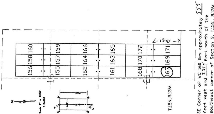
The above map depicts the WC 167 lode mining claim, which is located in Section (s) 21, Township 15 North, Range 13 West, Gila and Salt River Base Meridian, Mohave County, Arizona. The claim corners, end centers, and location monument are marked by 2 inch by 2 inch by 5 foot wooden posts with aluminum tags. The bearings and distances between claim corners are as depicted on the map.
