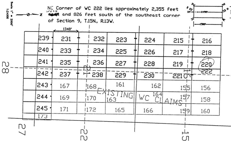
The above map depicts the WC 220 lode mining claim, which is located in Section (s) 16, Township 15 North, Range 13 West, Gila and Salt River Base Meridian, Mohave County, Arizona. The claim corners, end centers, and location monument are marked by 2 inch by 2 inch by 5 foot wooden posts with aluminum tags. The bearings and distances between claim corners are as depicted on the map.
