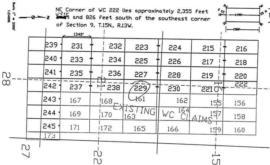
The above map depicts the WC 229 lode mining claim, which is located in Section (s) 21, Township 15 North, Range 13 West, Gila and Salt River Base Meridian, Mohave County, Arizona. The claim corners, end centers, and location monument are marked by 2 inch by 2 inch by 5 foot wooden posts with aluminum tags. The bearings and distances between claim corners are as depicted on the map.
