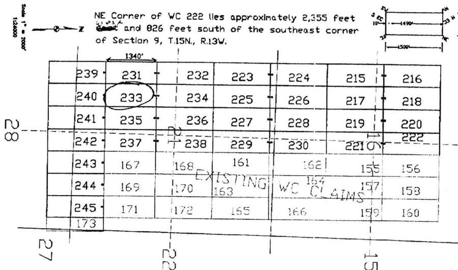
The above map depicts the WC 233 lode mining claim, which is located in Section (s) 21, Township 15 North, Range 13 West, Gila and Salt River Base Meridian, Mohave County, Arizona. The claim corners, end centers, and location monument are marked by 2 inch by 2 inch by 5 foot wooden posts with aluminum tags. The bearings and distances between claim corners are as depicted on the map.
