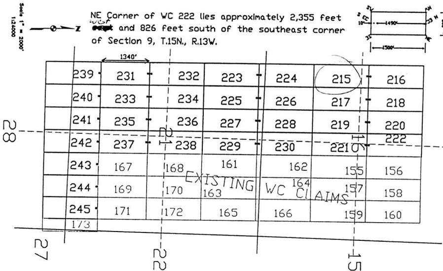
The above map depicts the WC 215 lode mining claim, which is located in Section (s) 16, Township 15 North, Range 13 West, Gila and Salt River Base Meridian, Mohave County, Arizona. The claim corners, end centers, and location monument are marked by 2 inch by 2 inch by 5 foot wooden posts with aluminum tags. The bearings and distances between claim corners are as depicted on the map.
