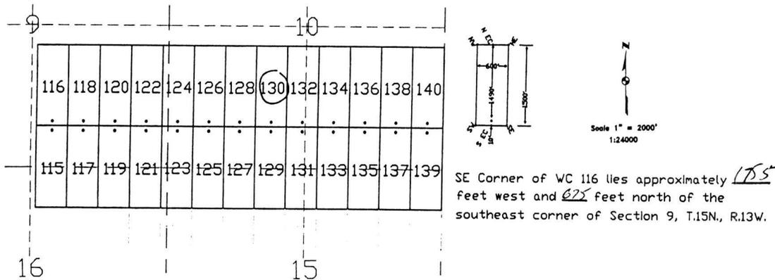
The above map depicts the WC 130 lode mining claim, which is located in Section (s) 10, Township 15 North, Range 13 West, Gila and Salt River Base Meridian, Mohave County, Arizona. The claim corners, end centers, and location monument are marked by 2 inch by 2 inch by 5 foot wooden posts with aluminum tags. The bearings and distances between claim corners are as depicted on the map.
