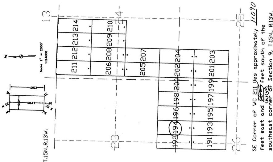
The above map depicts the WC 194 lode mining claim, which is located in Section (s) 20, Township 15 North, Range 13 West, Gila and Salt River Base Meridian, Mohave County, Arizona. The claim corners, end centers, and location monument are marked by 2 inch by 2 inch by 5 foot wooden posts with aluminum tags. The bearings and distances between claim corners are as depicted on the map.
