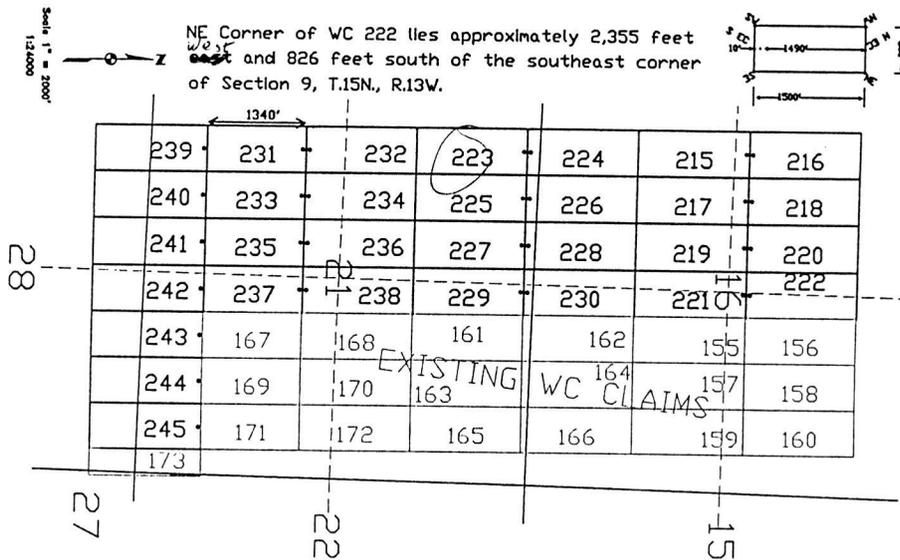
The above map depicts the WC 223 lode mining claim, which is located in Section (s) 21, Township 15 North, Range 13 West, Gila and Salt River Base Meridian, Mohave County, Arizona. The claim corners, end centers, and location monument are marked by 2 inch by 2 inch by 5 foot wooden posts with aluminum tags. The bearings and distances between claim corners are as depicted on the map.
