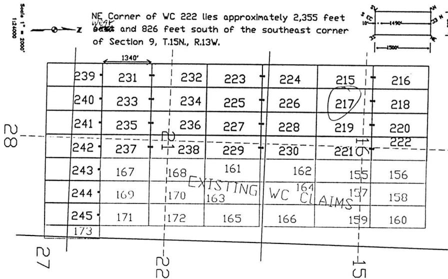
The above map depicts the WC 217 lode mining claim, which is located in Section (s) 16, Township 15 North, Range 13 West, Gila and Salt River Base Meridian, Mohave County, Arizona. The claim corners, end centers, and location monument are marked by 2 inch by 2 inch by 5 foot wooden posts with aluminum tags. The bearings and distances between claim corners are as depicted on the map.
