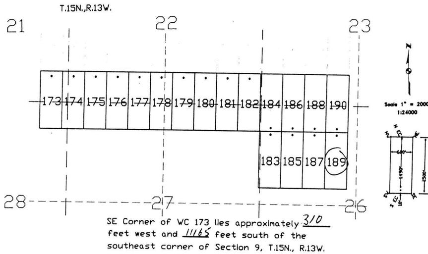
The above map depicts the WC 189 lode mining claim, which is located in Section (s) 26, Township 15 North, Range 13 West, Gila and Salt River Base Meridian, Mohave County, Arizona. The claim corners, end centers, and location monument are marked by 2 inch by 2 inch by 5 foot wooden posts with aluminum tags. The bearings and distances between claim corners are as depicted on the map.
