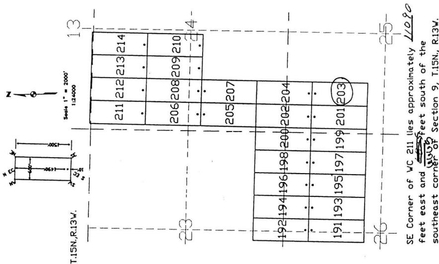
The above map depicts the WC 203 lode mining claim, which is located in Section (s) 25, Township 15 North, Range 13 West, Gila and Salt River Base Meridian, Mohave County, Arizona. The claim corners, end centers, and location monument are marked by 2 inch by 2 inch by 5 foot wooden posts with aluminum tags. The bearings and distances between claim corners are as depicted on the map.
