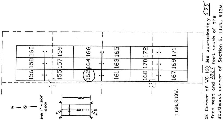
The above map depicts the WC 162 lode mining claim, which is located in Section (s) 16, Township 15 North, Range 13 West, Gila and Salt River Base Meridian, Mohave County, Arizona. The claim corners, end centers, and location monument are marked by 2 inch by 2 inch by 5 foot wooden posts with aluminum tags. The bearings and distances between claim corners are as depicted on the map.
