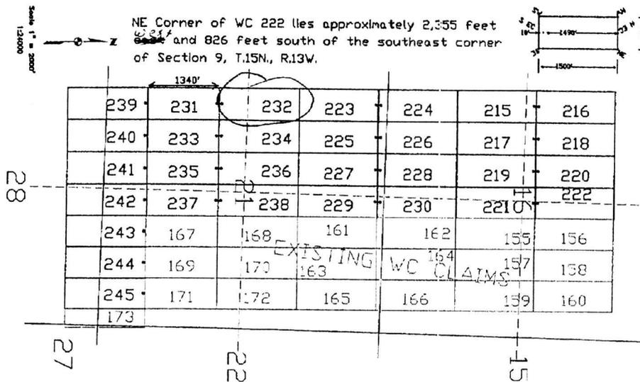
The above map depicts the WC 232 lode mining claim, which is located in Section (s) 21, Township 15 North, Range 13 West, Gila and Salt River Base Meridian, Mohave County, Arizona. The claim corners, end centers, and location monument are marked by 2 inch by 2 inch by 5 foot wooden posts with aluminum tags. The bearings and distances between claim corners are as depicted on the map.
