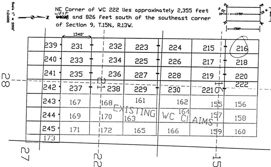
The above map depicts the WC 216 lode mining claim, which is located in Section (s) 16, Township 15 North, Range 13 West, Gila and Salt River Base Meridian, Mohave County, Arizona. The claim corners, end centers, and location monument are marked by 2 inch by 2 inch by 5 foot wooden posts with aluminum tags. The bearings and distances between claim corners are as depicted on the map.
