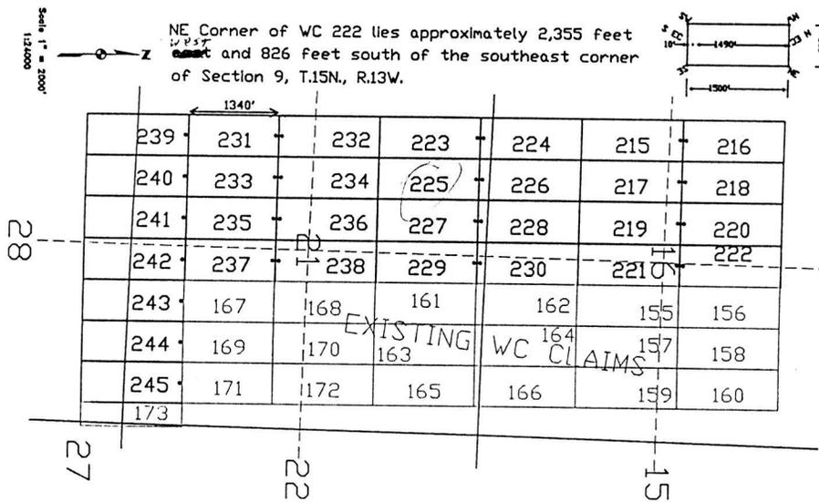
The above map depicts the WC 225 lode mining claim, which is located in Section (s) 21, Township 15 North, Range 13 West, Gila and Salt River Base Meridian, Mohave County, Arizona. The claim corners, end centers, and location monument are marked by 2 inch by 2 inch by 5 foot wooden posts with aluminum tags. The bearings and distances between claim corners are as depicted on the map.
