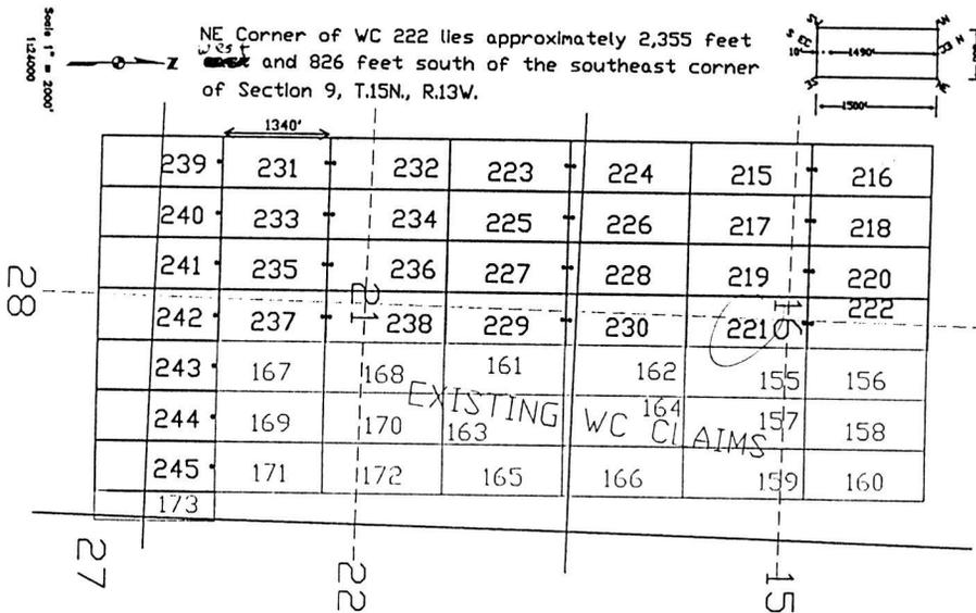
The above map depicts the WC 221 lode mining claim, which is located in Section (s) 16, Township 15 North, Range 13 West, Gila and Salt River Base Meridian, Mohave County, Arizona. The claim corners, end centers, and location monument are marked by 2 inch by 2 inch by 5 foot wooden posts with aluminum tags. The bearings and distances between claim corners are as depicted on the map.
