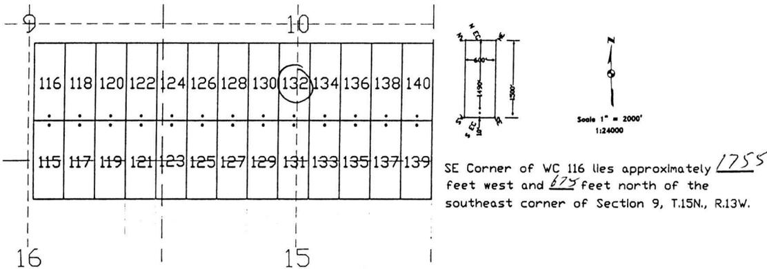
The above map depicts the WC 132 lode mining claim, which is located in Section (s) 10, Township 15 North, Range 13 West, Gila and Salt River Base Meridian, Mohave County, Arizona. The claim corners, end centers, and location monument are marked by 2 inch by 2 inch by 5 foot wooden posts with aluminum tags. The bearings and distances between claim corners are as depicted on the map.
