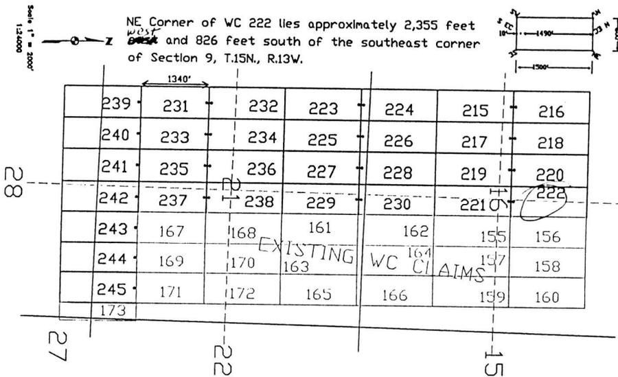
The above map depicts the WC 222 lode mining claim, which is located in Section (s) 16, Township 15 North, Range 13 West, Gila and Salt River Base Meridian, Mohave County, Arizona. The claim corners, end centers, and location monument are marked by 2 inch by 2 inch by 5 foot wooden posts with aluminum tags. The bearings and distances between claim corners are as depicted on the map.
