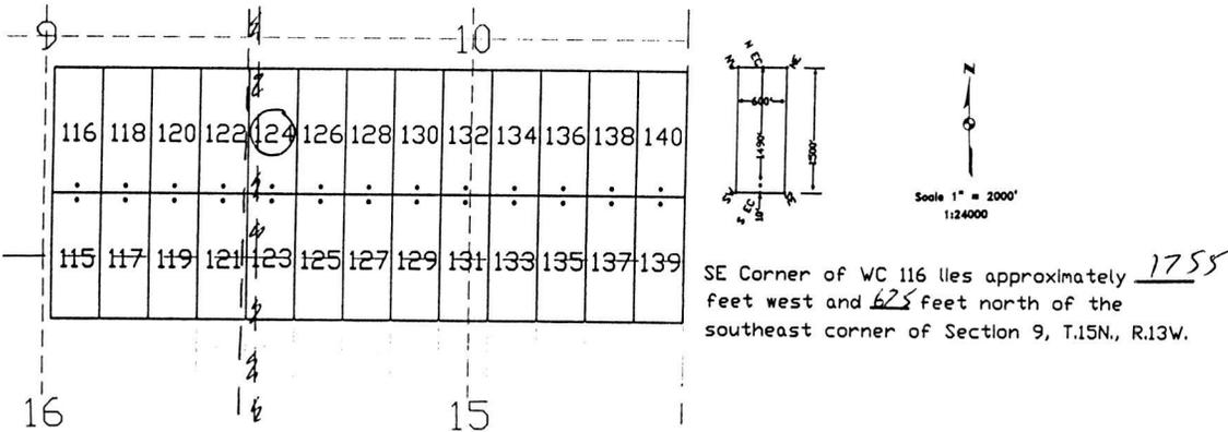
The above map depicts the WC 124 lode mining claim, which is located in Section (s) 10, Township 15 North, Range 13 West, Gila and Salt River Base Meridian, Mohave County, Arizona. The claim corners, end centers, and location monument are marked by 2 inch by 2 inch by 5 foot wooden posts with aluminum tags. The bearings and distances between claim corners are as depicted on the map.
