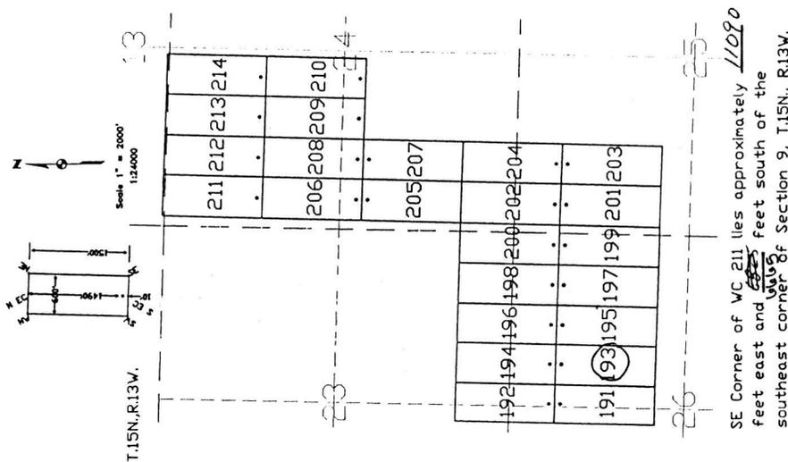
The above map depicts the WC 193 lode mining claim, which is located in Section (s) 26, Township 15 North, Range 13 West, Gila and Salt River Base Meridian, Mohave County, Arizona. The claim corners, end centers, and location monument are marked by 2 inch by 2 inch by 5 foot wooden posts with aluminum tags. The bearings and distances between claim corners are as depicted on the map.
