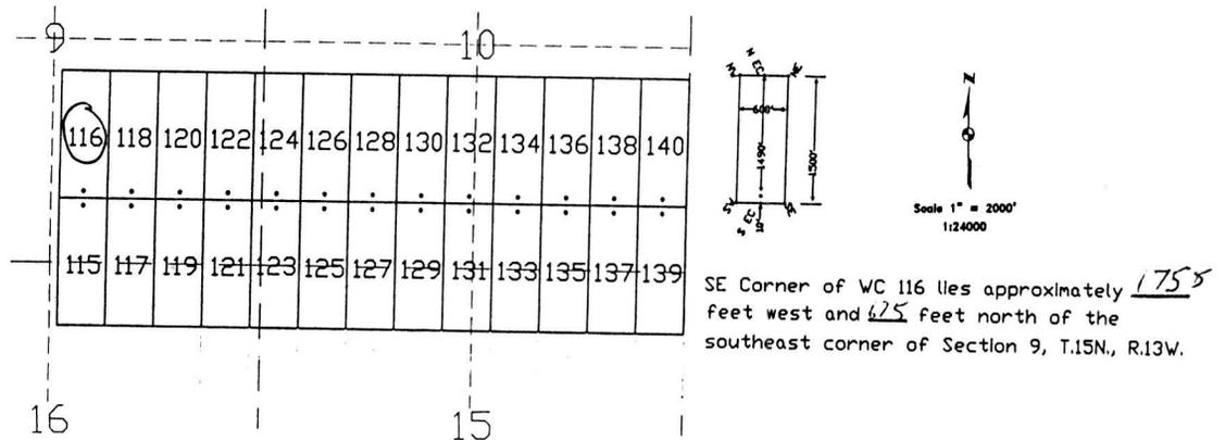
The above map depicts the WC 119 lode mining claim, which is located in Section (s) 9, Township 15 North, Range 13 West, Gila and Salt River Base Meridian, Mohave County, Arizona. The claim corners, end centers, and location monument are marked by 2 inch by 2 inch by 5 foot wooden posts with aluminum tags. The bearings and distances between claim corners are as depicted on the map.
