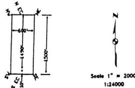
SE Corner of WC 153 is approximately 6045 feet east and 825 feet north of the southeast corner of Section 9, T.15N., R.13W.
